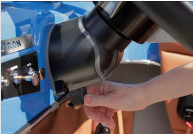
Tilt wheel standard All models excluding GTX
