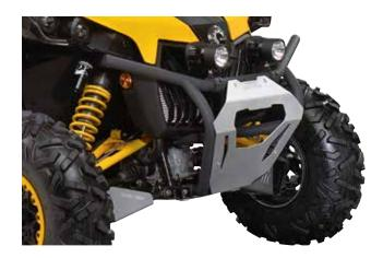
FRONT PRE-RUNNER BUMPER • Made of 1.5" (3.8 cm) diameter steel tube with a 1/8" (3 mm) aluminum plate for extra durability. Added heavy-duty protection in extreme conditions. • Mounting points for lights. • Requires Mounting Plate for Winch installation (715001699 or 705203196 for Maverick X mr). • Not EC compliant. Fits: RS
