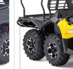
FLATBED PROTECTION TUBES • Bolt-on bumpers for the sides of the 6x6 flatbed. Protects the exterior plastic components of the flatbed from rocks, trees and other obstacles when traversing enclosed areas or loading cargo onto the bed. Fits: G2 (6x6 models only) 715002489 - Latin America / Asia Pacific 715002030 - Europe
