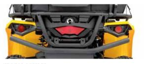
**XT REAR BUMPER** · Large tube construction. · Protects vehicle frame against the obstacles.
