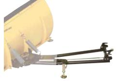
**ALPINE SUPER-DUTY** PUSH FRAME EXTENSION • 12 1/4" (31 cm) chassis extension for use with Apache 360 Track System. Increases angle and enables extra blade rotation. · Fits on Alpine Super-Duty Push Frame (715001063, 715001064, 715001182 & 715001474). 703500603
