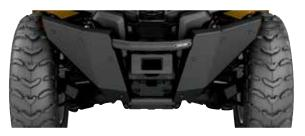
**EXTREME FRONT BUMPER** • Ultra-sturdy build. · Enhances front-vehicle protection. Compatible with XT Front Bumper. Fits: G2L 715002468
