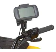
**GPS RAM®MOUNT FOR HANDLEBAR**  Convenient bracket for installing the Garmin Montana GPS (not included) onto your unit's handlebar. Fits: G2, G2L, G2S 715001985
