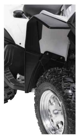
FENDER FLARE • Integrated extended Fender Flare for sporty look and full body protection from dirt and water. • Includes front and rear extensions and all mounting hardware. Fits: 62S (except X mr models) 715001681
