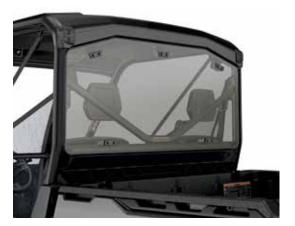
**REAR POLYCARBONATE WINDOW** • High-impact-resistant polycarbonate window. • Ideal for preventing backdraft of dust or rain in harsh environments.
