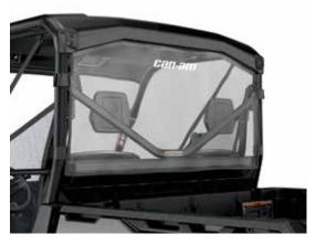
SOFT REAR WINDOW • Clear, flexible window made from transparent vinyl. • Resists cold-cracking to -4°F (-20°C). Fits: UR
