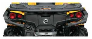
**XT REAR BUMPER** · Provides additional protection against the elements. • Tough and durable, can be added on base Outlander model to convert vehicle into XT model. · Large tube construction with textured black finish. • Standard on XT model. Fits: G2
