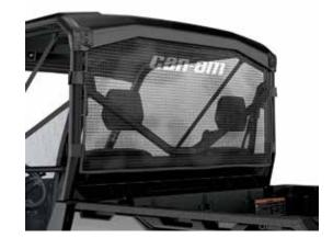
REAR WIND SCREEN • Black full rear mesh reduces windshield backdraft. • Roll-bar mounted. • Can-Am branded. Fits: UR 715002851
