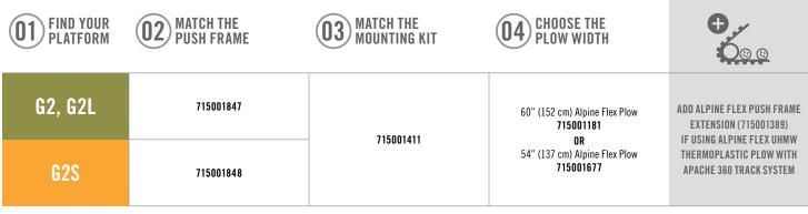
**ALPINE FLEX PUSH FRAME** WITH QUICK ATTACH SYSTEM • Refer to the chart on page 54 for the fitting. 715001848
