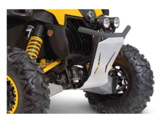
DUNE FRONT BUMPER • Made of 1.5" (3.8 cm) diameter steel tube with a 1/8" (3 mm) aluminum plate for extra durability. · Delivers additional heavy-duty protection in extreme conditions. · Features a more pronounced attack angle and mounting points for lights. • Not winch compatible. • Not EC compliant. Fits: RS 715001954 • Black
