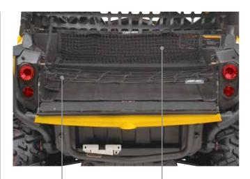
CARGO BOX ELASTIC NET • Elastic net designed to hook to the bottom of the cargo box. • Ideal for retaining lighter, irregular-shaped items. <u>Fits: RU</u> 715001372 • Black CARGO BOX STORAGE NET • Mesh net. • Stores items vertically. • Quick installation. Fits: RU 715001370 • Black
