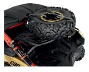
TUBE LinQ ADAPTOR - Cage mounted LinQ receiver. - Included in the LinQ Pivoting Rack assembly. - Allows the installation of single LinQ mounted accessories.
